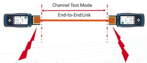
Failures due to field termination other than simple wire-map errors can not be found using Channel mode!
