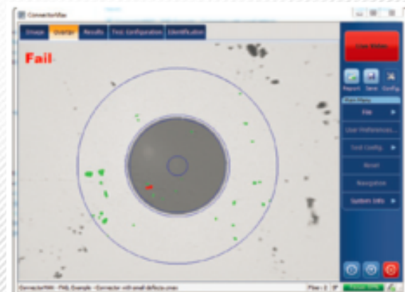
Defective connector failing acceptance criteria.
