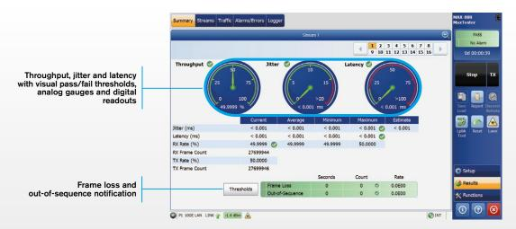
The analog gauges are lined with green and red layers to represent the expected thresholds.
