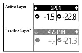
a. In a multi-layer PON, all downstream wavelengths from the OLT reach all ONTs. At service activation, when testing on the ONT side (any test point after last splitter), only one upstream wavelength is active, corresponding to the actual service activated.
