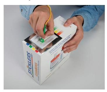
contamination onto the next connector. Once the cleaning process is complete, discard the wipe or swab and inspect the end-face to make sure all contaminants have been eliminated.
