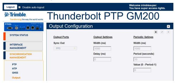
BNC Output: The type of output signal – PPS, PP2S, Periodic or 10 MHz
