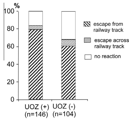
Fig. 5. Comparison of the reactions of roe deer to an oncoming train when the UOZ-1 device was on (+) or off (-) (chi-square = 9.9, df = 2 , p < 0.01 ). Sampling period was 33 and 19 months, respectively.
