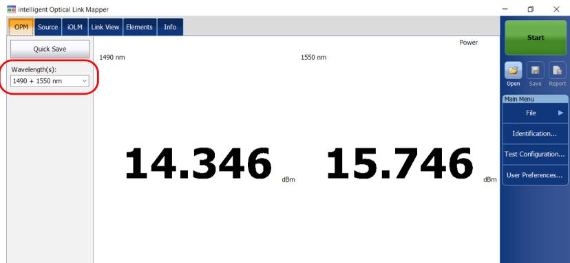
**Note:** *Two power levels are considered for measurement when two wavelengths are selected from the **Wavelength(s)** drop-down box.*
