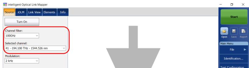
**Note:** If you have a DWDM or a CWDM module, the parameters set in the **iOLM** tab are applied automatically in the **Source** tab. See *Working With the DWDM Module* on page 59 or *Working With the CWDM Module* on page 69 for details.
