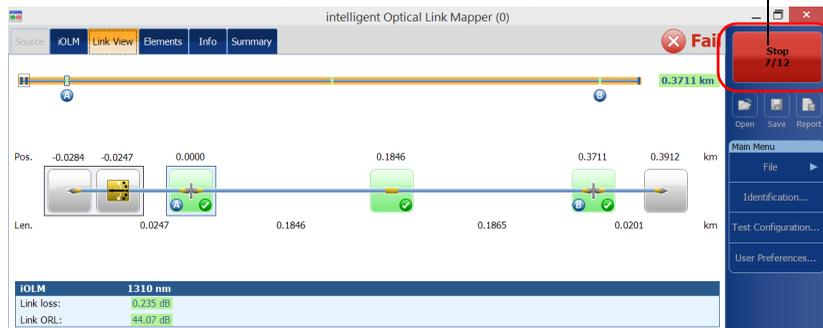
The stopped acquisition status will be saved in the measurement file. It is also displayed in the **Info** tab. See *Viewing Measurement Information* on page 188 for details.
