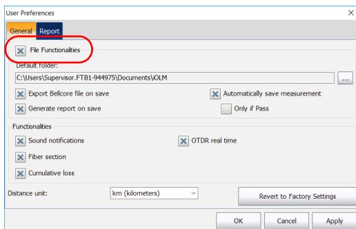
3. Select whether you want the measurements to be stored automatically regardless of the results, or only when the results have a pass status.
