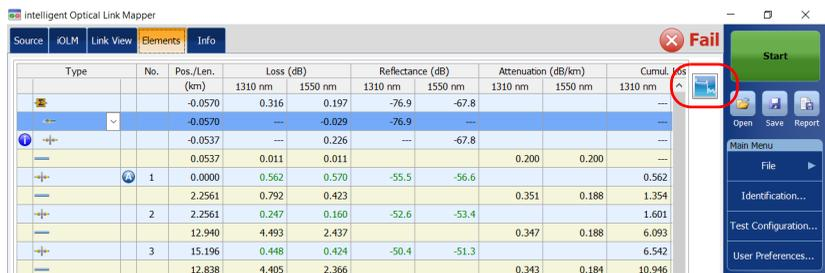
In the OTDR Viewer, you can navigate through the events or sections directly on the graph or in the event table.
