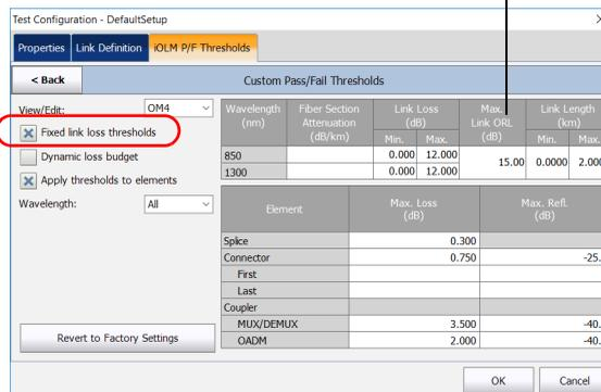
The screenshot shows the 'Test Configuration - DefaultSetup' dialog box with the 'Custom Pass/Fail Thresholds' tab selected. The 'Fixed link loss thresholds' checkbox is highlighted with a red circle. The dialog contains two tables: one for 'Link Loss (dB)' and 'Link Length (km)' for wavelengths 850 and 1300 nm, and another for 'Max. Loss (dB)' and 'Max. Refl. (dB)' for various elements.
