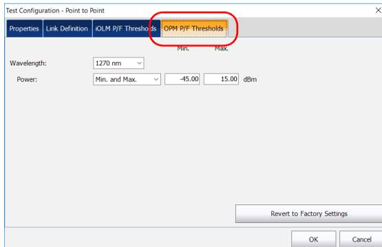
4. Enter the desired values for the minimum and maximum power, and select the wavelength for which the different pass/fail threshold values can be specified.
