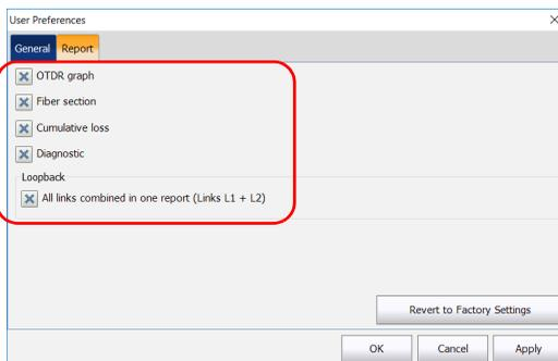
**Note:** The OTDR graph generation fails if the iOLM measurement does not contain the necessary intermediate OTDR data, if the iOLM acquisition process is interrupted by the user, or it is self interrupted because a live fiber is detected.
