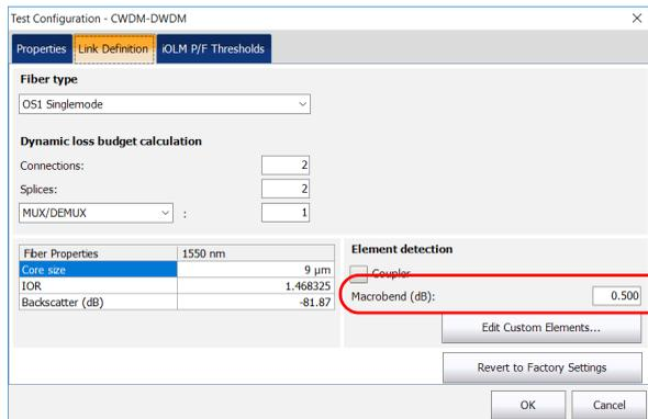
The screenshot shows the 'Test Configuration - CWDM-DWDM' dialog box. The 'Link Definition' tab is active. The 'Fiber type' is set to 'OS1 Singlemode'. Under 'Dynamic loss budget calculation', 'Connections' is 2, 'Splices' is 2, and 'MUX/DEMUX' is 1. The 'Fiber Properties' table is as follows:
