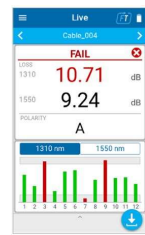
Power meter main screen
