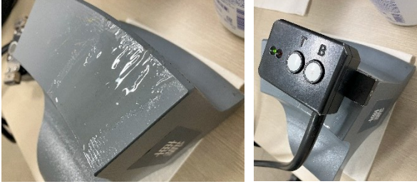
Fig.3 Ultrasonic couplant and probehead of the equipment.
