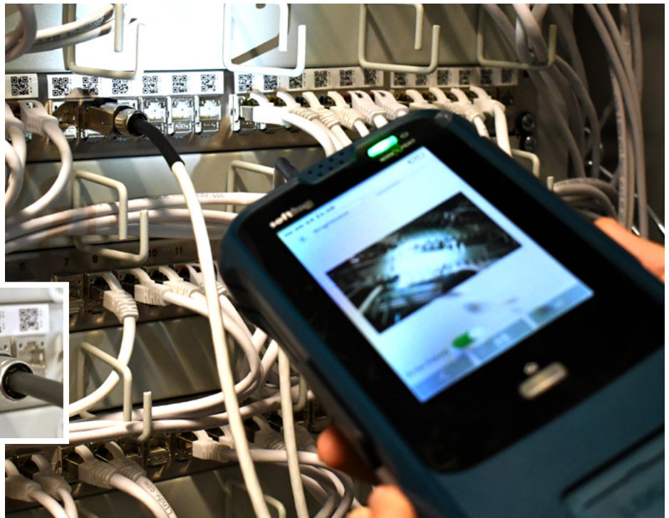
Before testing, scan the label with WireXpert MP
