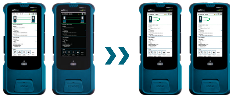
Setting for fiber optic loop testing
